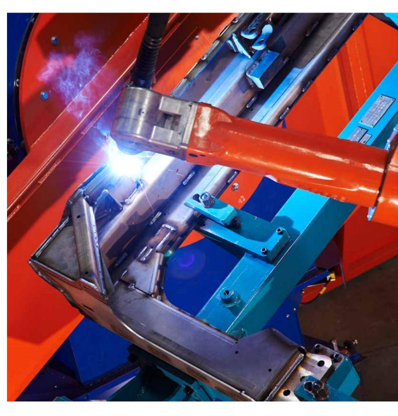
The **QIROX compact systems** are perfectly matched "ready to weld" systems in a compact size. Each compact system is equipped with two stations so that a high and economic duty cycle can be obtained. While the robot is welding the components on one side, loading or unloading is carried out simultaneously on the other station. Robot and positioner are mounted on a common base frame. This guarantees a quick and perfectly adjusted system assembly.
