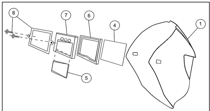
To insert the new outer protection **4** lens the filter must be removed by unscrewing the two retaining screws **8** from the inside of the helmet **1**.
